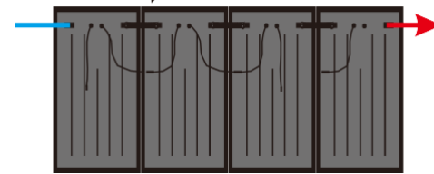
Simplified diagram installation of a hydraulic line with 4 panels in portrait
