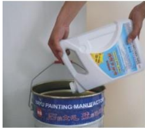
Pure water: 56% Original anti-freezing liquid: 44%
